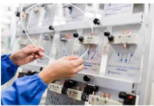
The components are mounted on modules that can be installed on a panel frame or a bench for teacher demonstration and student use.
